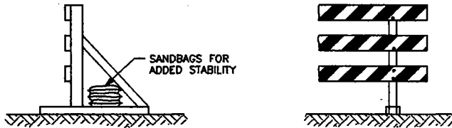
MOVABLE (TEMPORARY) TYPE III BARRICADE
